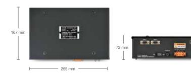
2 video channel input Analog RGB/Hs/Vs Up to 1920 by 1200 pixels Record interval 15sec/image Output to NDV-1900 via LAN Refresh rate 60 to 85 Hz Power 100V to 240V AC (15VA)
