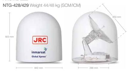
Downlink freq 19.2 to 20.2 GHz Uplink freq 29 to 30 GHz ICM: module iDirect (NTG-249) Block up convertor 5W Elevation range -20 to 115° Azimuth range 360° Temperature: -25° to 55°C
